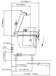
Cold Water inlet 1 (cleaning) CWII = Electrical inlet (power) ΕI
